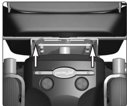
The two brackets are fitted with the seats rear fastening screws.
