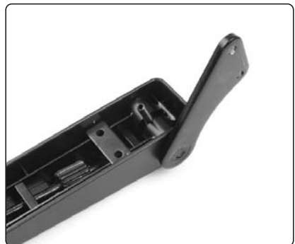
The armrest joint is refitted on the other side of the armrest.
