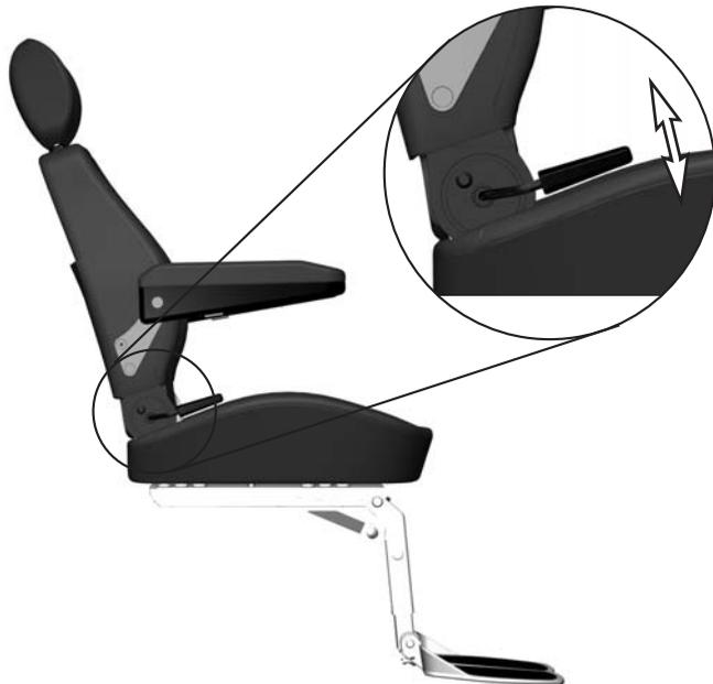
*The angle of the Backrest can be adjusted when the Backrest joint's release lever is pulled upwards.*
