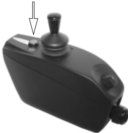
Figure 16. Main power switch
