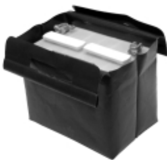
Figure 4. Acid batteries are placed in the battery case before being placed in the wheelchair.
