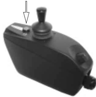
Figure 8. Main power switch
