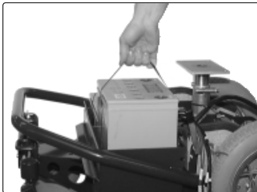
Figure 30. Using battery strap
