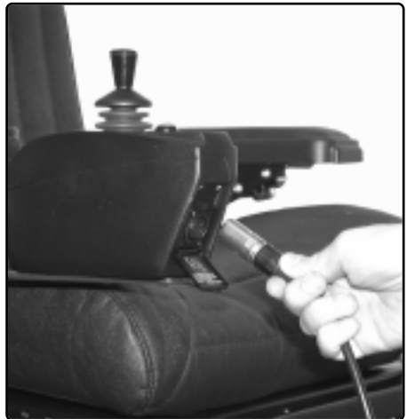
Figure 27. Charger connected to the charging socket.
