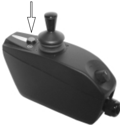
Figure 16. Main power switch
