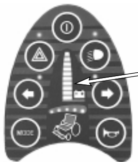
Fig.10. Battery voltage indicator
