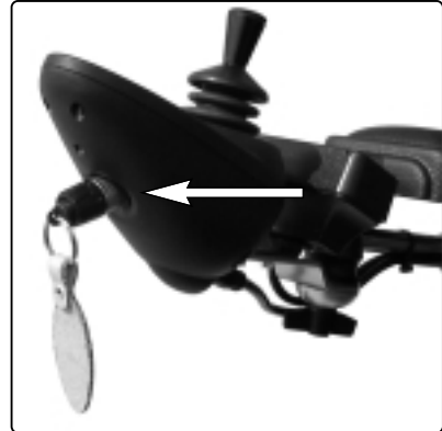
Panel outlet with security key
