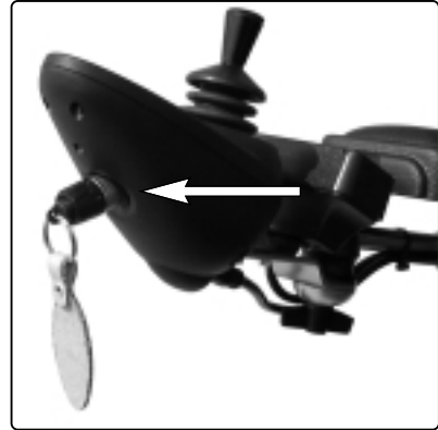
Panel outlet with security key
