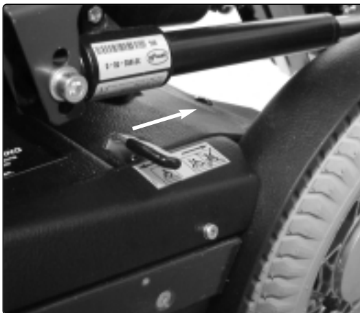
Figure 31. Releasing the brakes
