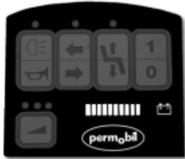
Figure 12. Battery voltage indicator
