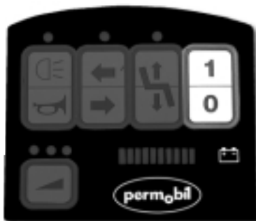
Figure 10. Main power switch
