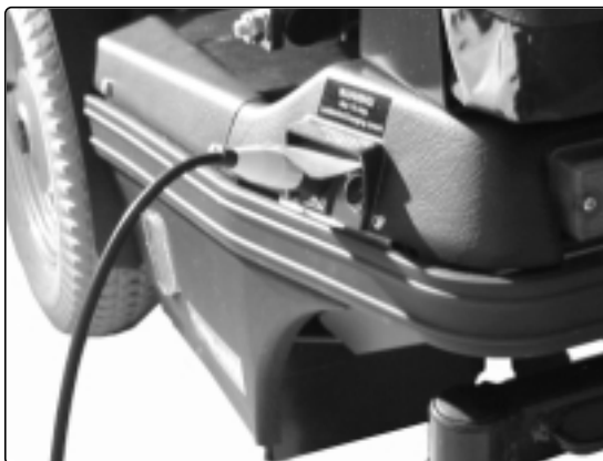
Figure 33. Connecting the charger
