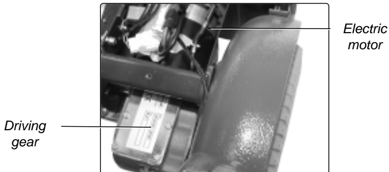
Fig.7. Electric motor with driving gear
