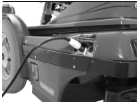
Fig. 38. Connecting the charger
