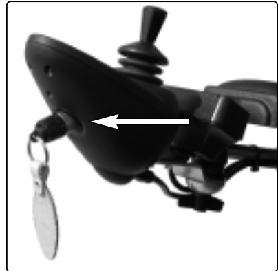
Fig. 11. Panel outlet with security key
