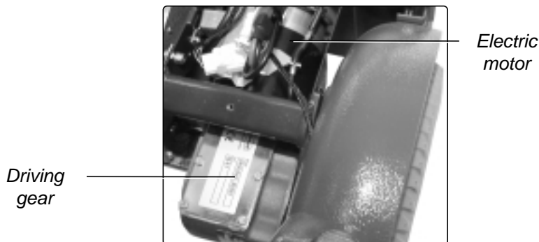
Figure 7. Electric motor with driving gear
