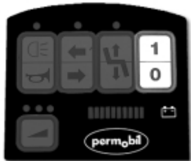
Figure 11. Main power switch
